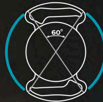
Imitation of contact angle of haptic against the capsular bag (diameter 10 mm) - 60°
