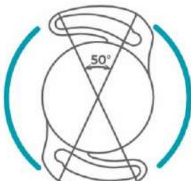
Imitation of the contact angle of haptic within the capsular bag (diameter-10 mm) - 50°
