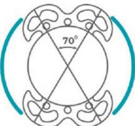
Imitation of the contact angle of the haptic within the capsular bag (diameter-10 mm) - 70°
